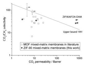
Figure 4. CO<sub>2</sub>/CH<sub>4</sub> separation performance of the present ZIF-90 mixed-matrix membranes, compared with the compiled data on MOFcontaining mixed-matrix membranes. [15-18,25] Data marked by \* is based upon our mixed-gas permeation measurements. Data from previous work marked with \*\* carries a large error bar owing to inaccuracy in measuring low permeabilities. [25] The upper bound for polymer performance as defined in 1991 is shown.
