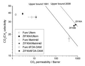
Figure 3. Gas-permeation properties of mixed-matrix membranes containing 15 wt% of ZIF-90 crystals measured with pure gases. Measurements were performed at 35 °C and 4.5 atm upstream pressure for Ultem and Matrimid membranes, and at 25 °C and 2 atm upstream pressure for 6FDA-DAM membranes. The data for pure Ultem and Matrimid are averaged values from the literature. [13b, 24] The upper bounds for polymer membrane performance as defined in 1991 and 2008 are shown.
