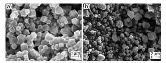
Figure 1. SEM images of submicrometer-sized ZIF-90 particles; a) ZIF-90A synthesized using methanol as a nonsolvent; b) ZIF-90B synthesized using deionized water as a nonsolvent.
